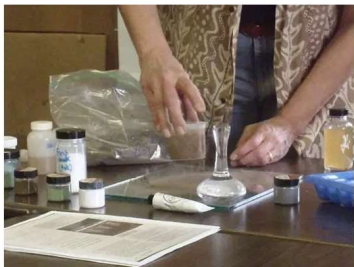
Demonstrating the muller for making paint
